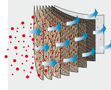
Multi-layer filter mats consist of superimposed layers of paper. The large number of openings lets air pass virtually unhindered.
