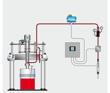
Connection diagram for a metering system with switchgear cabinet, electrically operated ball valve, material pressure regulator, volume meter and metering valve. Two-hand operation of the dual-post drum ram maximizes safety. Fluid level sensors can also be fitted.
