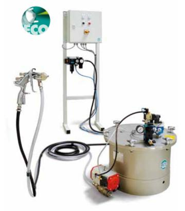
Easy Flow works entirely without pumps and is therefore particularly suitable for use with shear-sensitive adhesives. The pressure tank is refilled automatically when the fluid level is down to a minimum. A maximum of 10 workstations can be supplied with material. Supply lines may be as much as 25 m long.
