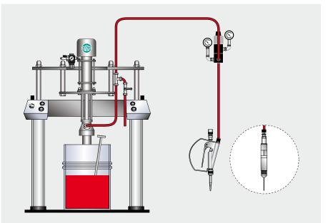
Connection diagram for a supply and application system for viscous materials. Manual and automatic valves are available. Two-hand operation of the dualpost drum ram maximizes safety. Fluid level sensors can also be fitted.
