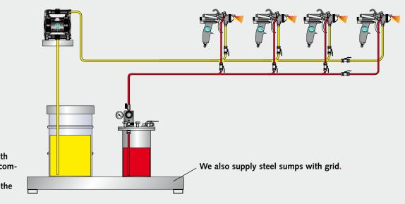
System design with pumps for the A component and MDG pressure tank for the B component
