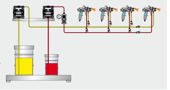
System design with pumps for both components. A material pressure regulator is available for the B component.
