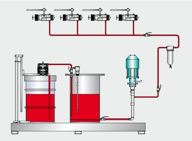
Shipping containers and process containers for continuous material delivery. We also supply steel sumps with grid.
