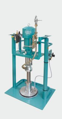
Pump unit with dual-post ram for 20 to 60 liter drums
