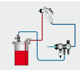
Model with separate filter and pressure regulator
